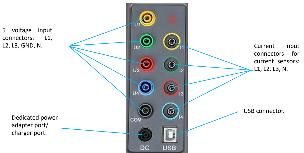
Figure 3-3: Connectors on the top of device
